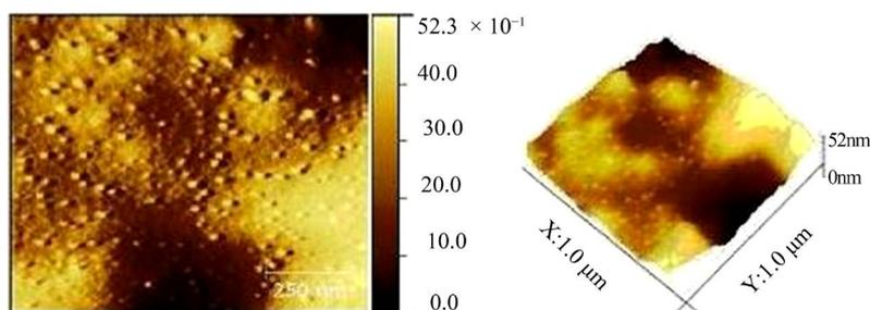
**Figure 2.** AFM pattern of neem synthesized silver nanoparticles.
