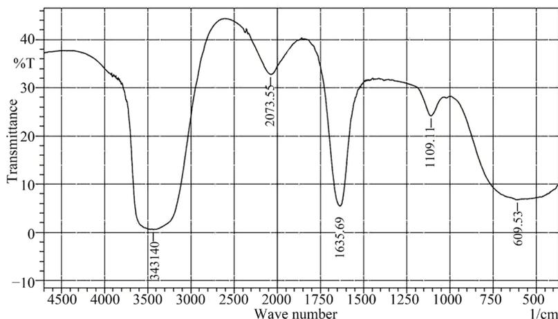
**Figure 3.** FTIR pattern of neem synthesized silver nanoparticles.
